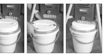
5. Place the lid onto the bucket (b). Press down on the lid (c) and slide the bucket under the feed guide (h).
